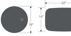
Fixed Height Surface Model Code: PLT-TF/-BTF will **not** have a thumb button in the surface.
